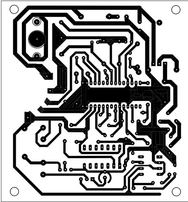
Fig. 4: Actual-size, single-side PCB of noise-muting FM receiver
