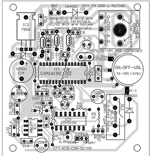
Fig. 5: Component layout for the PCB
