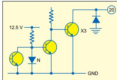
Fig. 2: Internal circuit schematic around pin 20 of CXA1619S
