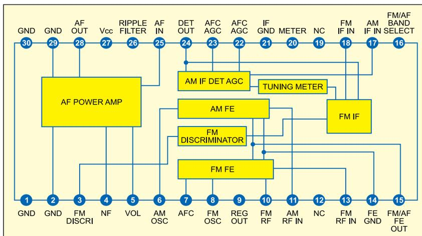
Fig. 1: Functional block diagram of Sony CXA1619S
